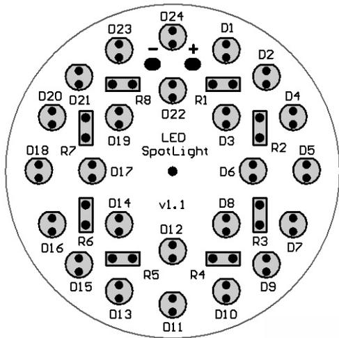
The design of the **LED SpotLight** allows for all 24 LEDs (located at **D1** to **D24**) to be powered from the common power input area just below **D24**.
