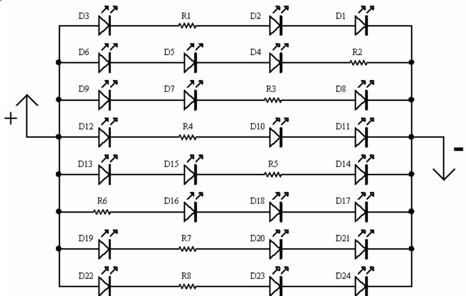
The schematic shows the LEDs wired in sets of three with each set having its own current limiting resistor. A full 24 LEDs running on the board will draw a total of approximately 160mA.
